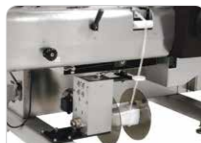
Longitudinal trim sealing system rewind for polyolefin shrink films
