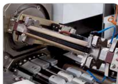
"D-Cam" type cross sealing jaw system
