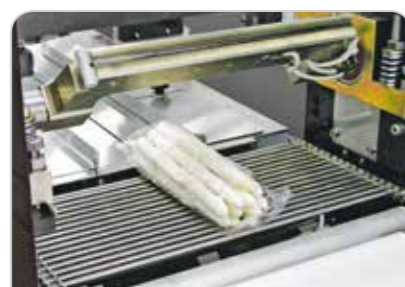
Motorized carrier through the sealing jaws
