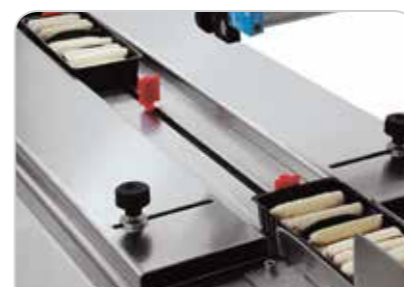
Photocell control for "No Product - No Bag" function
